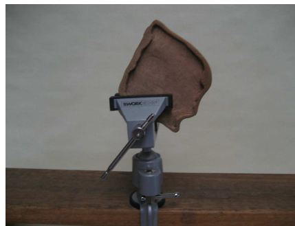
Soft rubber jaws stops damage to work
