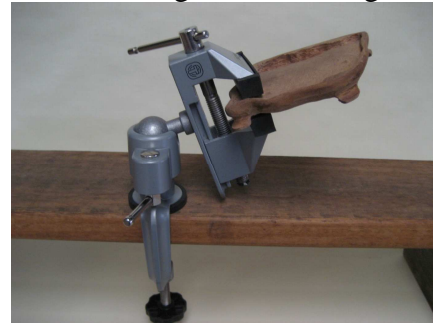
Rotates through 360 x 45 degrees horizontally and 90 degrees vertically
