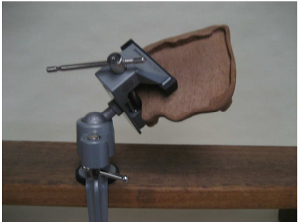
Rotates through 360 x 45 degrees horizontally and 90 degrees vertically
